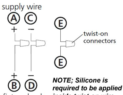
**NOTE:** Silicone is required to be applied inside twist-on wire connectors to make a water tight seal.
